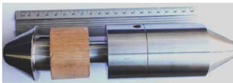
Figure 3 – The borehole probe
