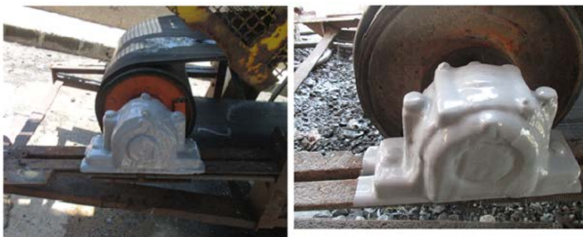
Figure 7: Later application of thermoplastic polymer on the different bearings.
