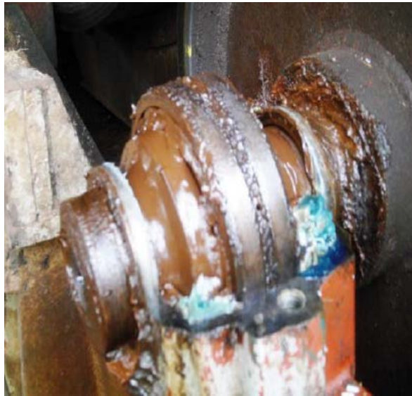
Figure 8: Bearing in regular operating conditions without protection with less than 6 months of use. Note how contaminated the grease becomes.
