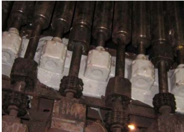
Figure 4: Later application of thermoplastic polymer on the bearings.
