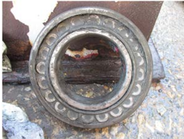
Figure 5: Bearing without protection with high level of contamination by dust and moisture.
