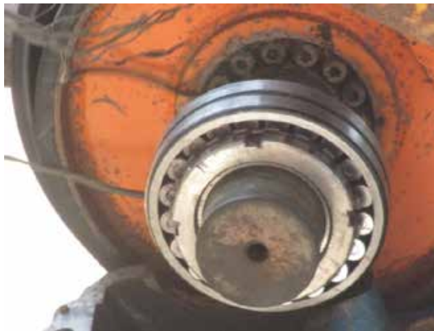
Figure 6: Bearing after washing and placed on shaft.
