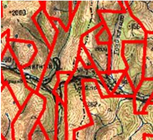
Figure 4. Third order faults between blocks with different orientations of rose diagrams of stripes
