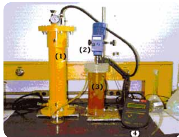
Photo 23. Bench-based dissolved air flotation unit. (1) Saturator, (2) mechanical stirrer, (3) flotation cell, V = 2, 0 \text{ L} , (4) pH meter
