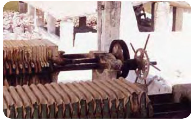
Photo 26. Filter press to produce pie residues with high solid content
