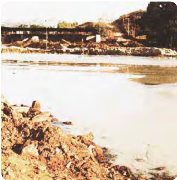
Photo 59. A tank for final disposal of the waste from the sawing of ornamental rock blocks
