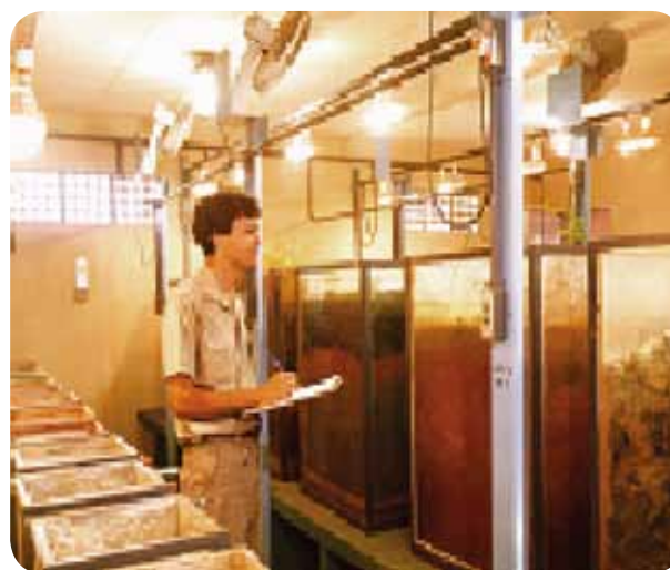
Photo 22. AMD laboratory with lysimeters in Rio Paracatu Mineração
