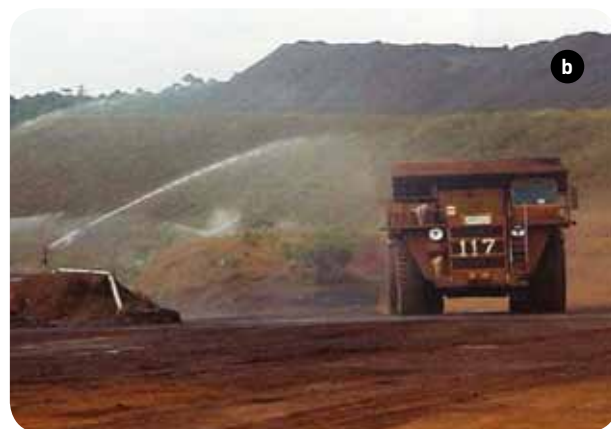
Photo 8 (a and b). Water used to control dust emission. Source: MBR
