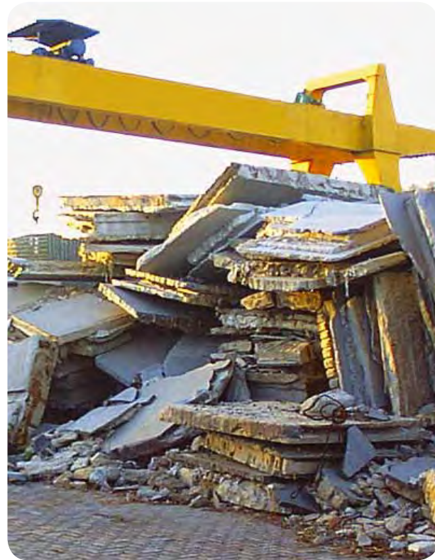
Photo 65. First and last “slice” from the sawing of blocks on a bandsaw
