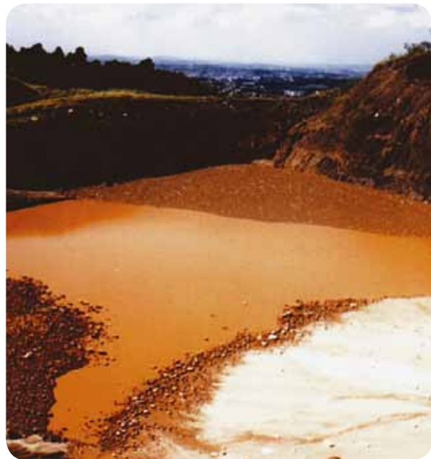
Photo 85. Sump and settling tank for rainwater, including sediments retained
