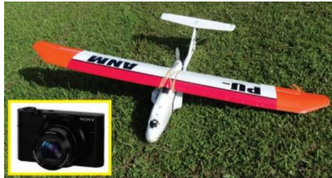
Figure 1 – \mu UAV developed by UnB in partnership with DNPM. In detail, non-metric camera, model DSC-RX100, used to obtain the air photos.
