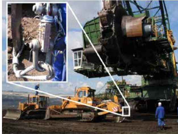
Figure 6 – Mass release with use of the special device (Czmochowski, 2008)
