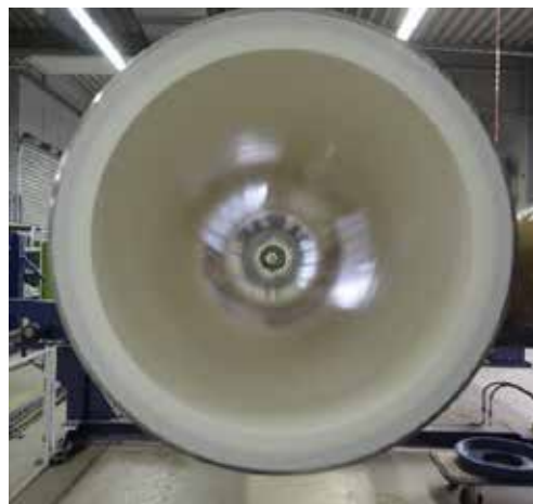
Figure 3: Internally coated pipe for oil sands hydrotransport
