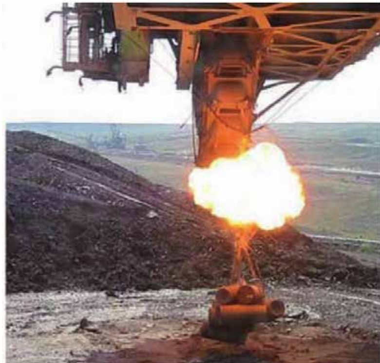
Figure 7 – Mass release with use of explosives (Gottvald, 2010)
