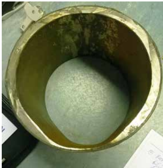
Figure 1: Abrasive wear on steel pipe
