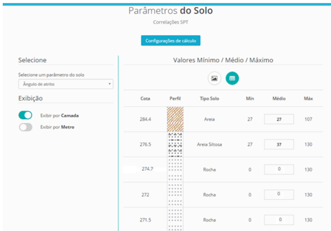
Figure 6 – Representative profile of the probe into the hole indicated with the average values of the soil parameters by layer
