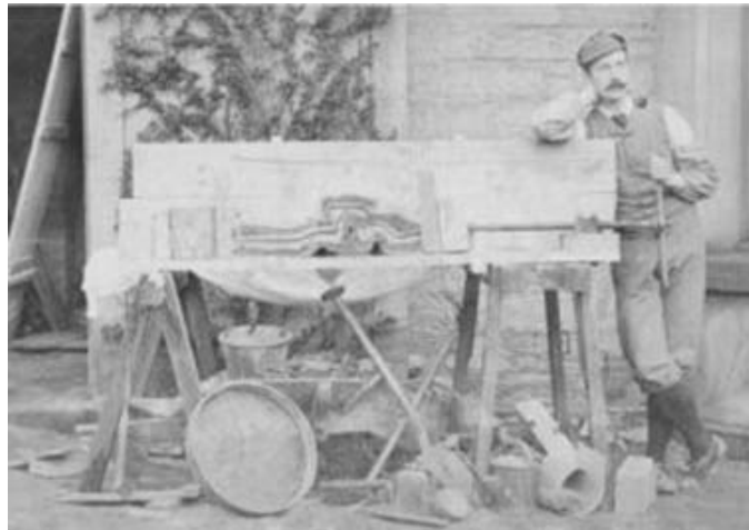
Figure 1 – Photograph of Cadell and his thrusting analogue experiments (source: Geological Survey of Great Britain's Memoir).
